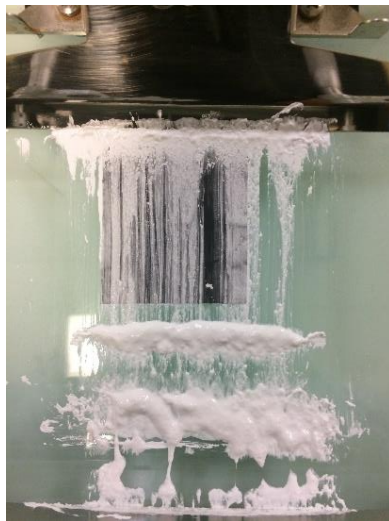
Figure 3.3. Slurry of A14325 grade alumina powder coated on LTO with 50 \mu\text{m} blade gap.
